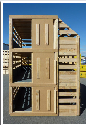
A three tier upper deck livestock pen. The dished carpet can be seen inside the open sliding doors.
