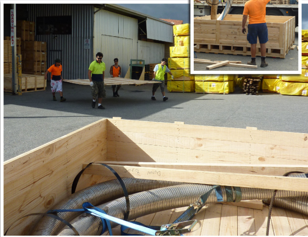
The 1.6 tonne hose secured in its custom built wooden crate, with the lid about to be lifted into place.
