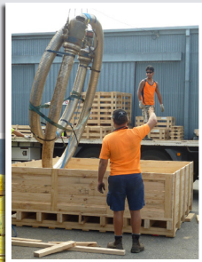
The 1.6 tonne hose being lifted into the custom built wooden crate.
