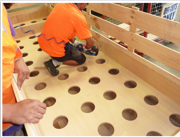
One of the custom built wooden crates showing the plywood internal fitout.
