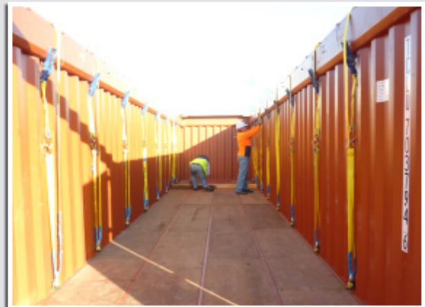
The ratchets straps are being secured in the empty sea container so the bore casings can be loaded.
