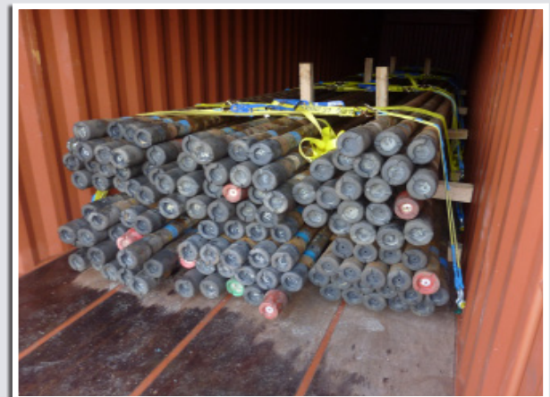
The bore casings secured with the ratchet straps and dunnage inside the sea container.
