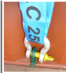
Left: The ratchet strap cable tied to the top bull-ring. Right: The shackle combination used to eliminate pinching.
