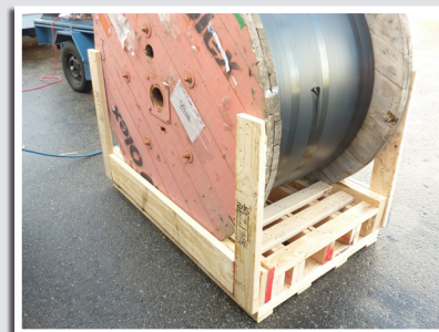
The cable drum on the reverse base pallet with all the lateral and vertical timber dunnage pieces attached.
