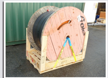
The cable drum fully secured to the modified reverse base pallet with timber dunnage and ratchet straps in place.
